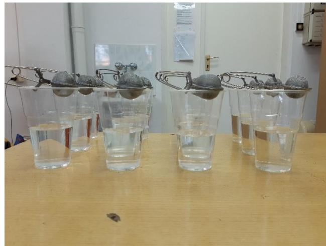
**Figure S2.** Water absorption test for crushed pellets from the WS blend with the addition of CS.
