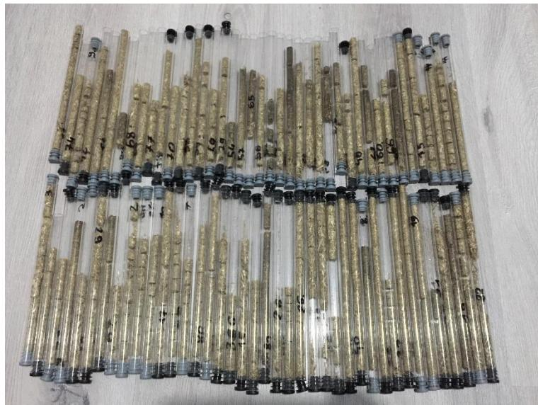
Fig. S2. An exemplary photo of pellets made of the blend of WS and CS at different technical parameters of compaction: material moisture content, die height, material temperature, and additive ratio
