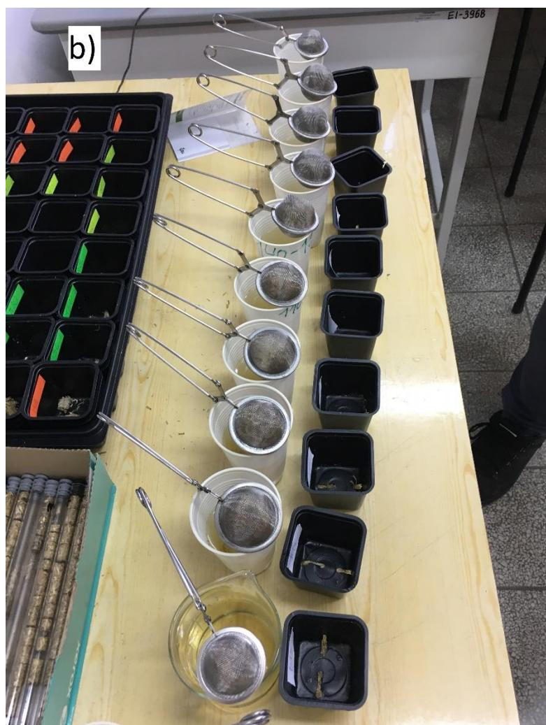
Fig. S2. Stands for measuring pellet quality parameters a) pellet strength during tensile strength, b) water absorption by uncrushed and crushed pellets
