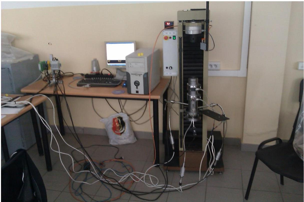
Fig. S1. Stand for biomass compaction with a single matrix with an open chamber, using a universal testing machine, as well as a system for controlling and recording parameters of compaction process
