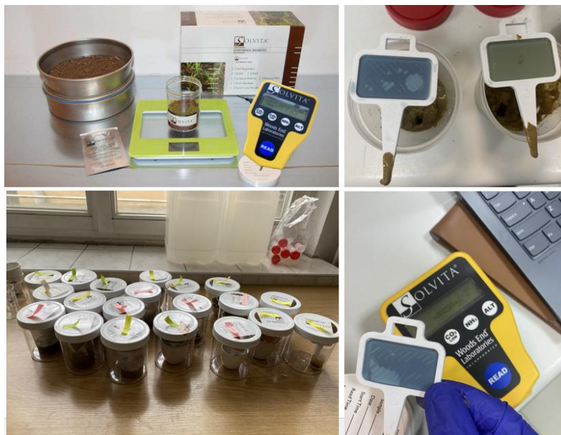
Figure 5.14. Preparation of soil samples for respiration measurement using the SOLVITA® Digital Color Reader.
