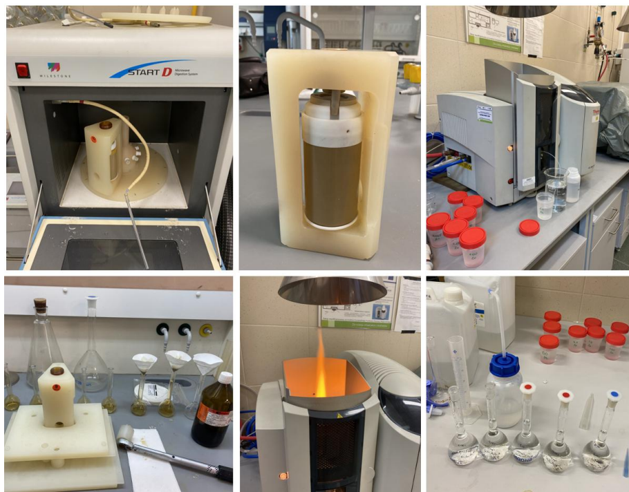
Figure 5.8. Mineralization of soil samples and determination of HMs content, from left – mineralization, from right – determination of metals by AAS (own photos).
