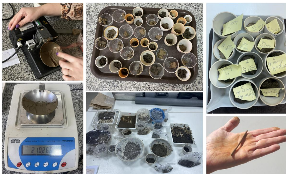
Figure 5.7. Determination of plasticity and liquidity of the tested soils (own photograph).
